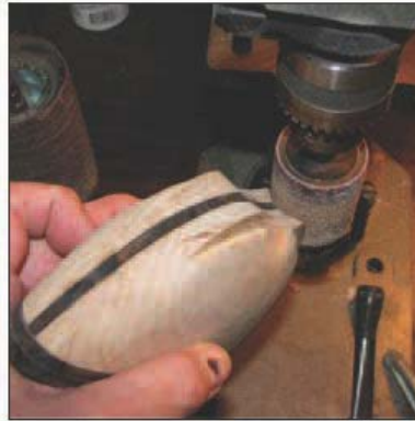
Figure 7 Use sanding to finalize shape.
