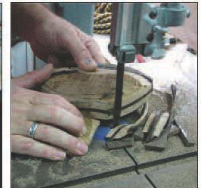
Figure 5 Rough bandsaw the feet & form.
