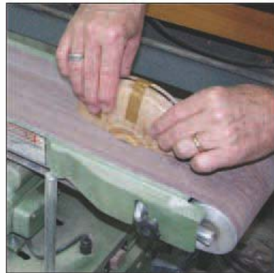
Figure 8 Level the vessel top glue joint.
