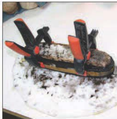
Figure 9 Segments form the top on a mold.
